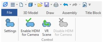
In addition, VR headset management commands are available for Camera objects created by user in the 3D model.
