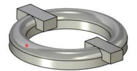
To blend only one part of the model, you need to select an auxiliary point. Only the closest to the given point faces will be blended.
