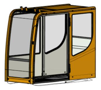
The geometry of the cabin can be uploaded to a separate file so that several users can work in parallel. To do this, a fragment is created in the context of the assembly, and reference elements are unloaded into it.
