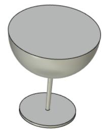
After selecting the removed face, the shell will be built for the entire body, and not just for its spherical part.
