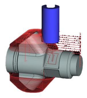
Example of combination of turning and milling on multi-axis turning center.
