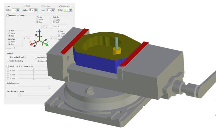
Predicts part overcutting and collision of the cutting tool with fixtures and working bodies of the machine.
