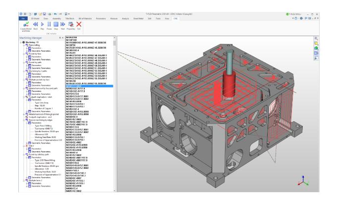
T-FLEX CAM is a fully integrated manufacturing add-on to T-FLEX CAD for generating NC programs as well as toolpath verification and machine simulation with material removal. provides comprehensive machining tools for a broad spectrum of manufacturing sectors.
