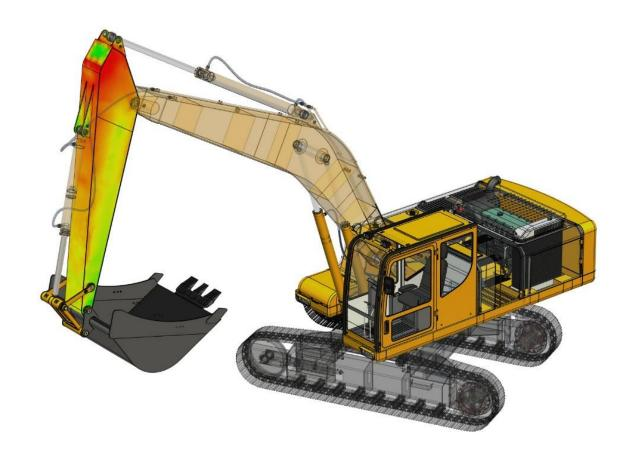
T-FLEX Analysis offers a wide spectrum of powerful tools to help engineers to perform virtual testing and analysis for predicting the physical behavior under various loading conditions.
